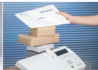
Differential weighing saves time by calculating the exact postage for each item removed from the weigh platform
